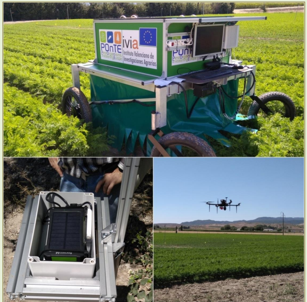
Fig. 10. Robotic platform for Calsol surveys.
